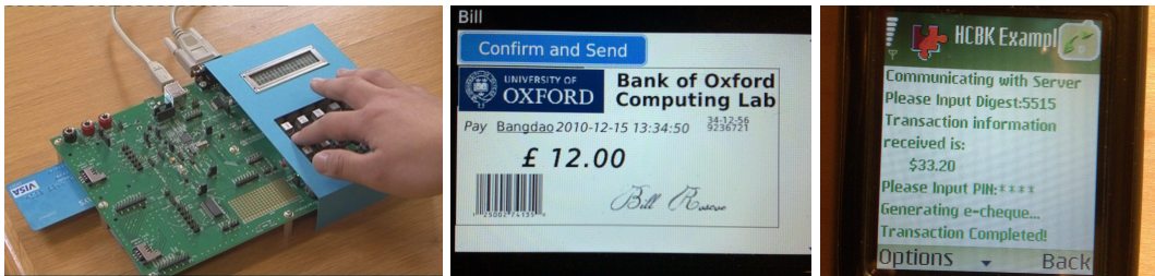
Fig. 2. Demonstrations: SD with card reader, phone-to-phone, phone-to-server (from left to right).
