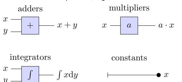
GPAC can solve any ordinary differential equation – extensions can do more functions
